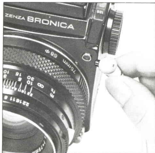
B. Always use flash cords with a standard PC type plug.
